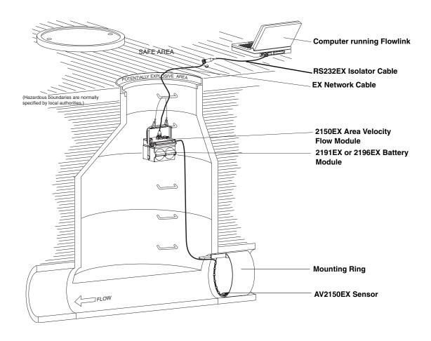
Figure 2-1 Typical Round-pipe Installation Connected to a Laptop Computer (Portable Installation, see section 2.4)
